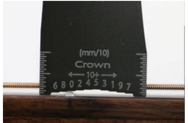
Fret crown height gauging (mm/10) This is same function as Step Gauge (see page 41).
