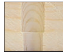
Cross section of drilled hole
