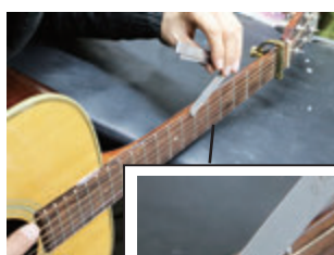
Checking a relief of the neck
