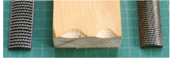
Comparison between CP file and normal wood file
