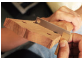
Checking flatness for installing machine heads
